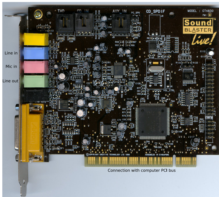
Figure 3.3.: A typical sound card.
